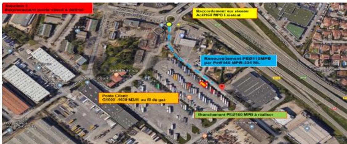
Figure 7 : Raccordement PE $\varnothing$ 160 – Etude raccordement GRDF 2018
